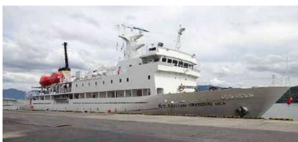
M/V Kapitan Gregorio Oca (Delivery : 25 th December 2018 at Miho Shipyard JPN) Length over all : 78.60m Breath Molded : 12.00m Draft Molded : 4.99m Gross Tonnage 2,980 tons
